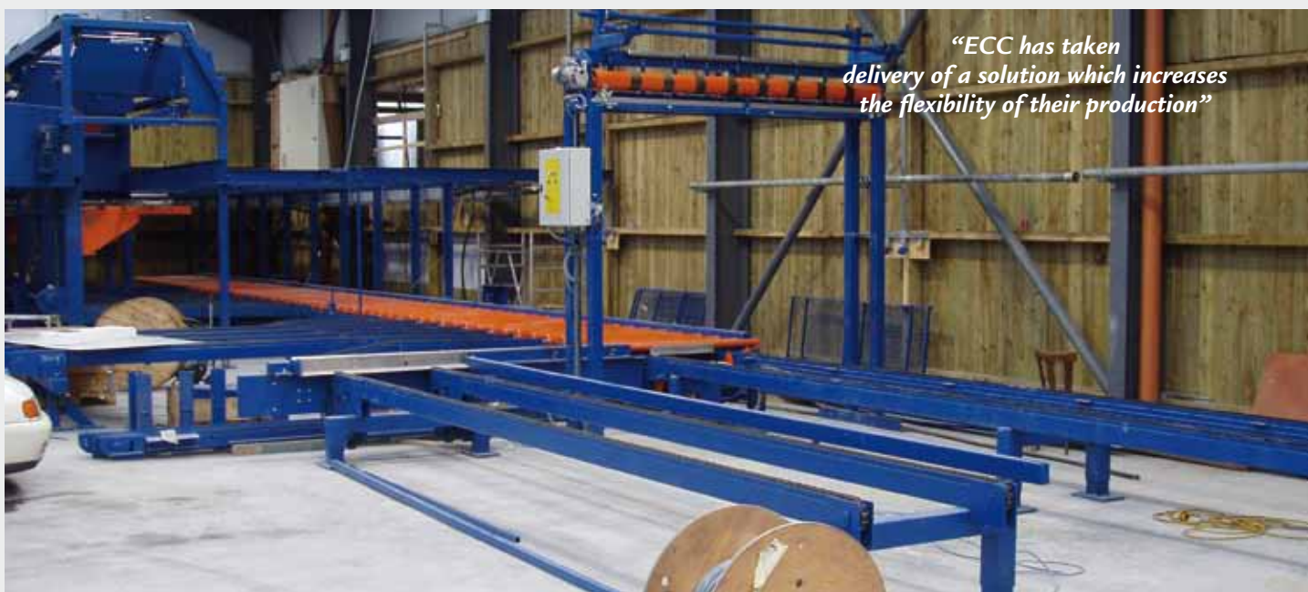
Assembly of a line for transporting packs through film-wrapping, automated bearer insertion and strapping
